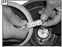
Make sure to connect the plug from remote to the plug coming from fan body according to the arrows indicated on the plugs, otherwise the remote will be damaged.
